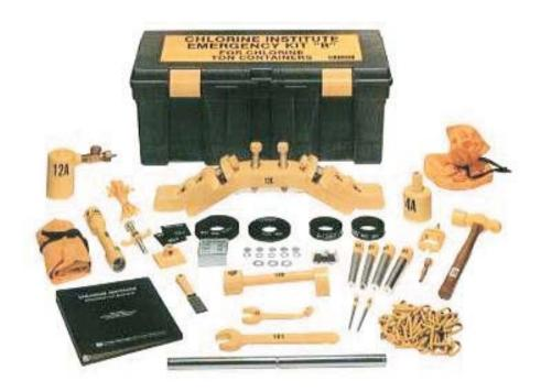
The Chlorine Institute Emergency Kit "B" is manufactured to the design specifications of the Chlorine Institute. The Emergency Kit "B" contains devices to stop leaks at the valves, fusible plugs, and in the side wall of chlorine one ton containers which conform to specification DOT 106A500X. Two instruction booklets explaining the application of each device are included. An instruction video for Kit B is also available.
